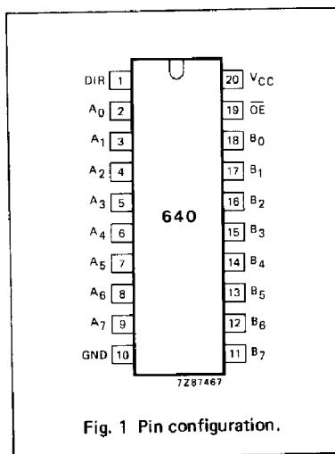
Fig. 1 Pin configuration.
