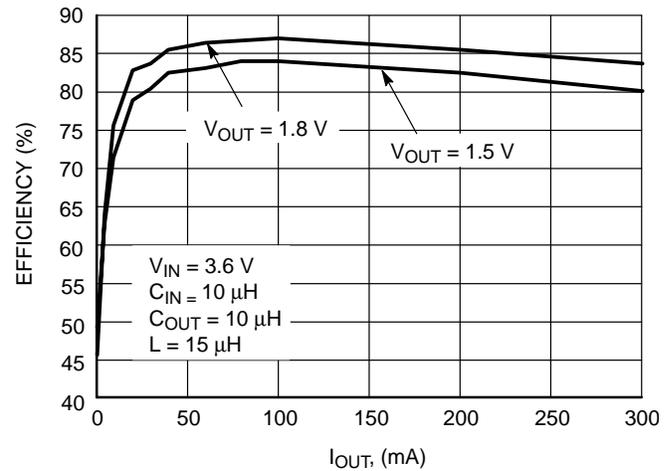
**Figure 11. PWM Efficiency**
