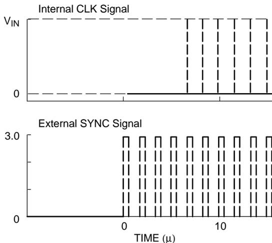
Figure 3. Timing Diagram of the SYNC Signal
