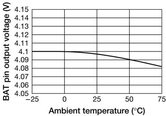
■ Re-charge detection voltage – Temperature
