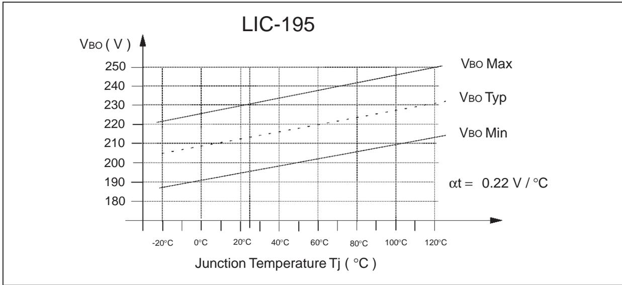
**VARIATION OF  $V_{BO}$  VERSUS JUNCTION TEMPERATURE**
