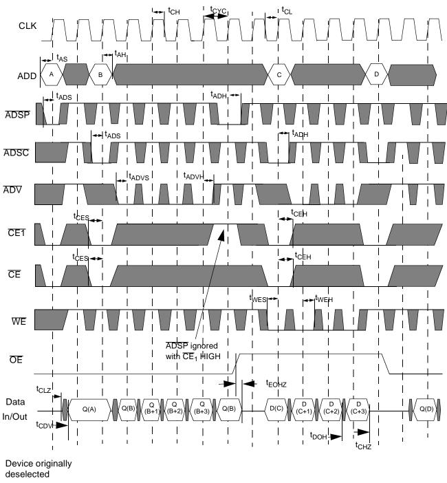
WE is the combination of BWE,  $BW_{[3:0]}$ , and  $\overline{GW}$  to define a write cycle (see Cycle Description Table). CE is the combination of  $CE_2$  and  $\overline{CE}_3$ . All chip selects need to be active in order to select the device. RAx stands for Read Address X, WAx stands for Write Address X, Dx stands for Data-in X, Qx stands for Data-out X
