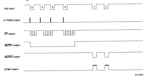
After the pulse dialing (including IDP) has completed, when DTMF key input operations are performed, DTMF signals are output continuously while keys are pressed.
