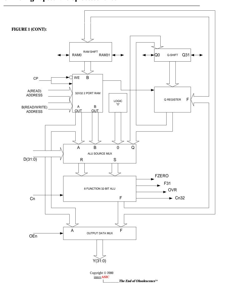
A detailed block diagram for the IA59032 is shown in Figure 1. The two key elements in the block diagram are the 32 word by 32-bit 2-port RAM and the high-speed ALU.
