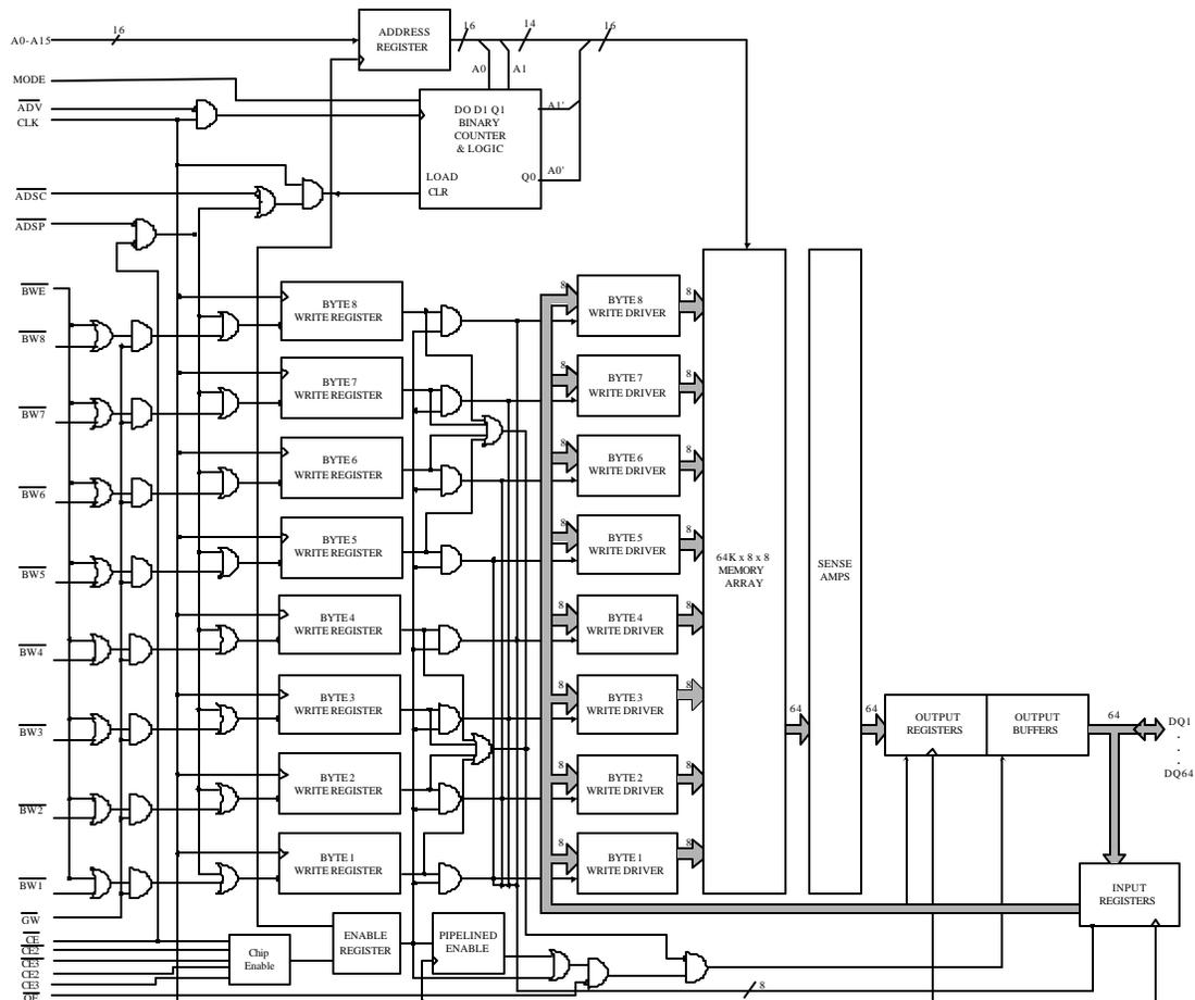
**Note:** The Functional Block Diagram illustrates simplified device operation. See Truth Table, pin descriptions and timing diagrams for detailed information.
