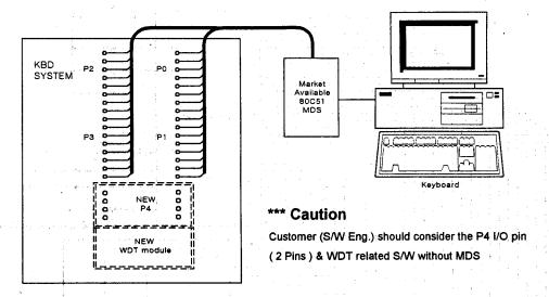
2. Second Stage: Target System Emulation with Adapter B/D which including EVA Chip and EPROM
