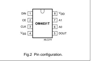
The OM4031T digital post-detection filter oversamples the noisy binary data stream at input DIN (pin 1), and outputs a noise-reduced data stream via open-drain output DOUT (pin 5). The filter bandwidth can be doubled to ease the search for bit synchronization on the data output signal.
