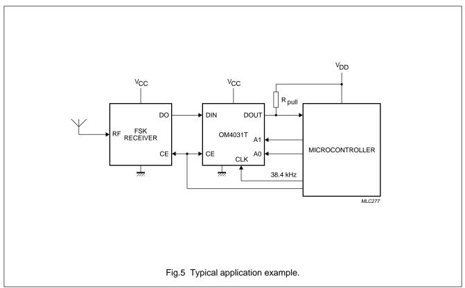
The OM4031T will generally operate from the same power supply ( $V_{CC}$ ) as the FSK data receiver providing its input data. The open-drain data output allows level shifting of the data to suit a microcontroller operating at a higher power supply voltage ( $V_{DD}$ ).
