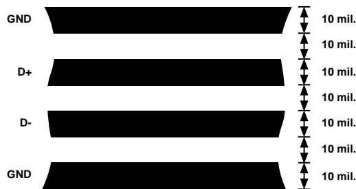
Figure 19. Arrangement of Signal Tracks
