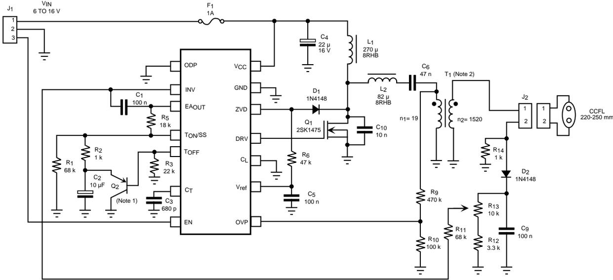
Gen. Note: Q<sub>2</sub> is not required if Q<sub>1</sub> is an avalanche rated FET
