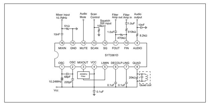
In the above application circuit, the audio signal is recovered using a conventional quadrature FM detector. The absence of an input signal is indicated by the presence of noise above the desired audio frequencies. This "noise band" is monitored by an active filter and a detector. A squelch trigger circuit indicates the presence of noise (or a tone) by an output which can be used to control scanning. At the same time, an internal switch is operated which can be used to mute the audio.
