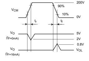
$$CM_H = \frac{160(V)}{t_{\Gamma}(\mu s)}, CM_L = \frac{160(V)}{t_{\Gamma}(\mu s)}$$
